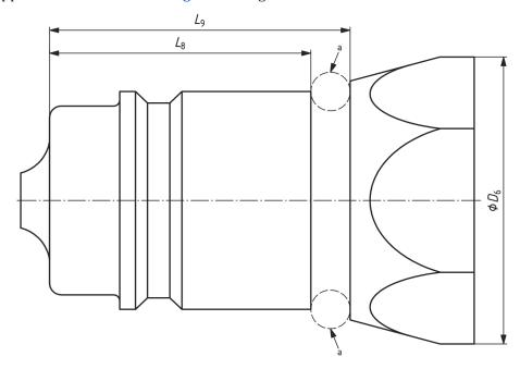
Shape of neck between  $L_8$  and  $L_9$  is optional but shall be circular to accommodate dust sealing.
